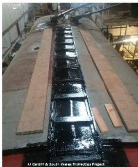
Picture showing walkways with timber cross-members all painted in bitumastic.
