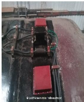
Picture Showing the front cowls fitted & the radio suppressor box.
