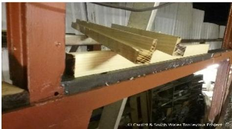
The two main window pillar uprights, clearly showing the "L" shape to fit the body pillars
