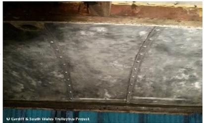
That's better the new aluminium strips in place showing the coach bolt fasteners to good effect.
